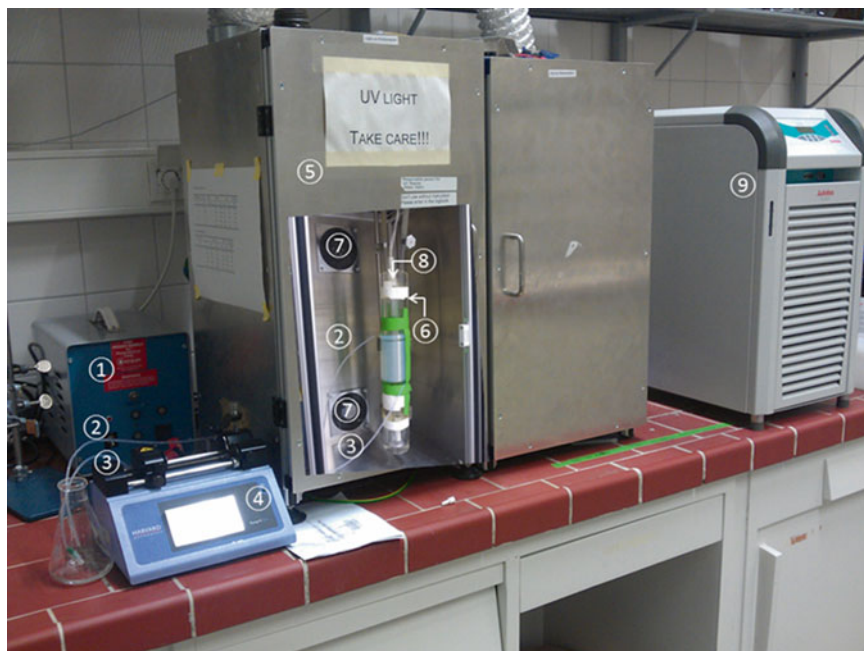
Fig. 2 Continuous-flow photoreactor. (1) 450 W Power supply; (2) FEP tubing inlet connected to disposable syringe on a syringe pump (4); (3) FEP tubing outlet; (5) UV box fitted with two fans (7); (6) a quartz glass cooling system connected to a chiller (9); (8) UV filter (Pyrex, 50 % transmittance at 305 nm)
